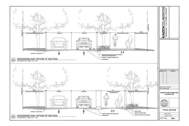
Option "A" shows a trail with a five foot landscape buffer that would accommodate new trees. The existing trees along Woodward Way would need to be removed in order to construct this trail option. The proposed replacement trees would be a four inch caliper tree and are part of the tree recompense plan that is before the City Park Arborist.
